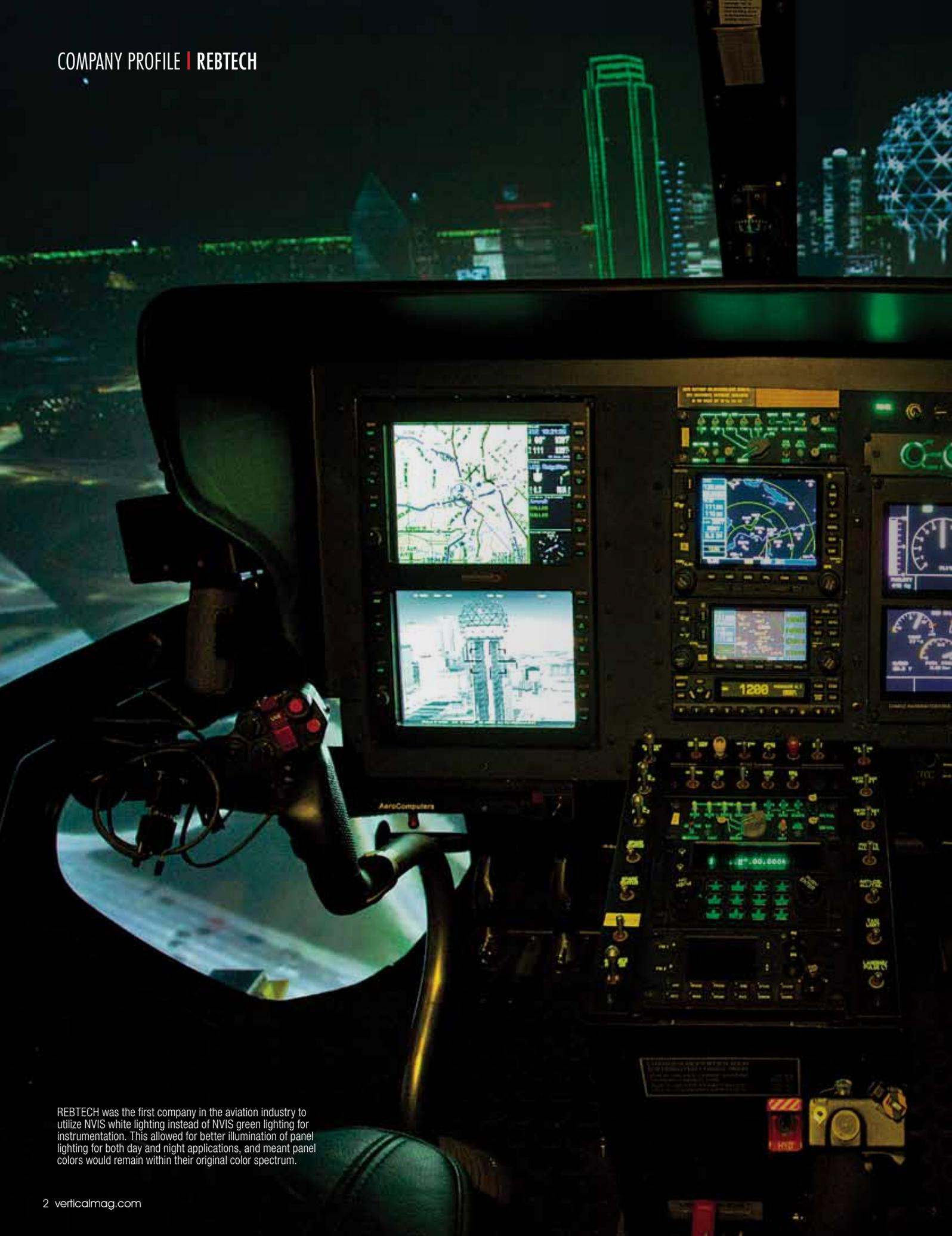
REBTECH was the first company in the aviation industry to utilize NVIS white lighting instead of NVIS green lighting for instrumentation. This allowed for better illumination of panel lighting for both day and night applications, and meant panel colors would remain within their original color spectrum.
